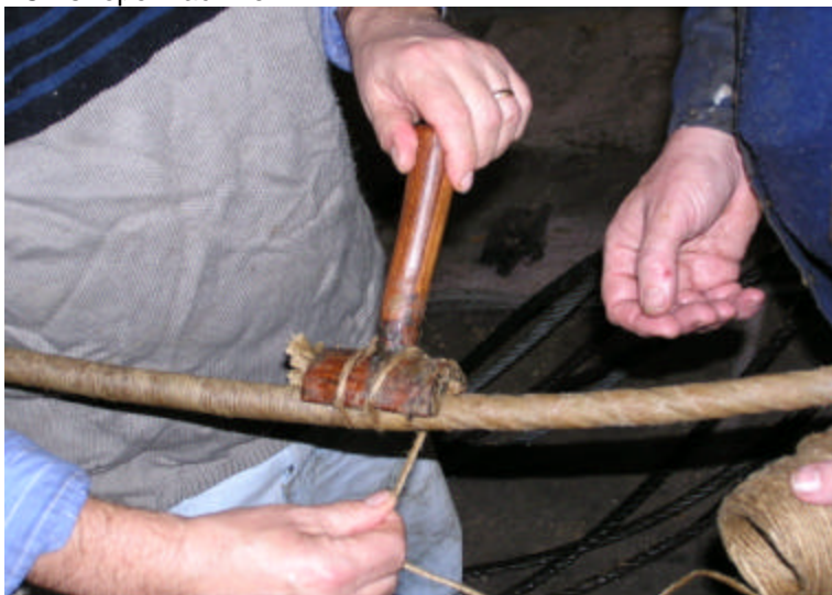
FCB and a mate serving some of the May Queen's standing rigging.
